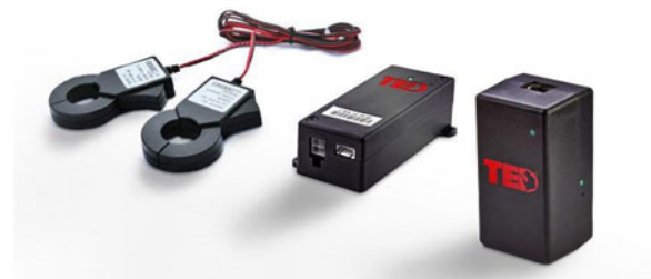
Fig. 6 The TED 5000G, including (left to right) one set of current clamps and measuring transmitting unit for breaker panel installation, and one gateway to transmit data externally
